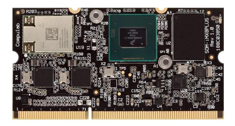
CL-SOM-iMX8-Plus is a tiny Computer-on-Module (CoM) built around the NXP i.MX8M-Plus. It features high performance graphics and image capabilities for a wide range of applications which require high-speed graphics including industrial HMI, medical, IOT, digital signage and professional audio visual devices.
